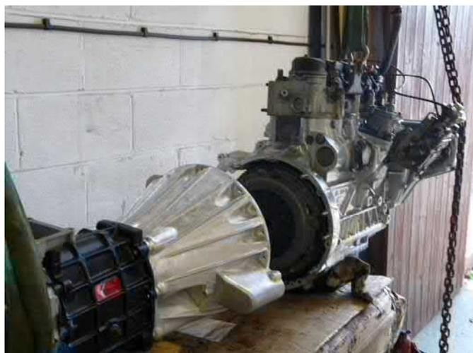
First of all, the engine was drained of all the oil. I'd left this in as protection more than anything else. The engine was stripped of all the ancillaries and thoroughly cleaned, jet washed after a coating with engine degreaser, then another coating of degreaser and hand cleaned. After that it was out with the rotary wire brushes. I bought some micro wire brushes from Ebay to get into all the little crevices, which worked well. It was then a wash down with a paint cleaner before painting.
