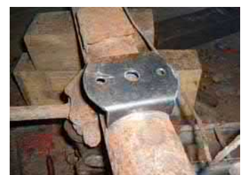
New mount ready for welding.
